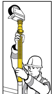
Turn the base the correct way up with the wheels on the ground. Use a spirit level to check the base unit is level. Adjust the legs as necessary, to level the base unit.
