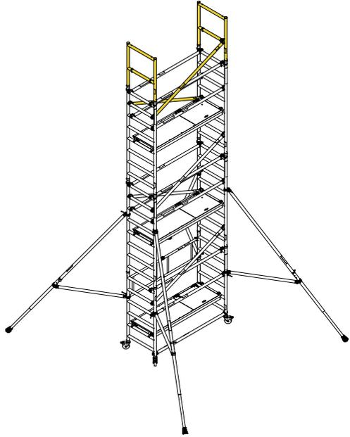
**10** Reposition trapdoor decks and horizontal braces.
