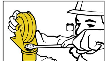
Follow the instructions in the adjustable leg pack to change the large castor spigot to the smaller one supplied in the pack. Insert the new castor into an adjustable leg and then retighten the fixing bolt with the spanner, following the instructions. Repeat this process for the other castors and adjustable legs. Insert the four leg and castor assemblies into the base unit.
