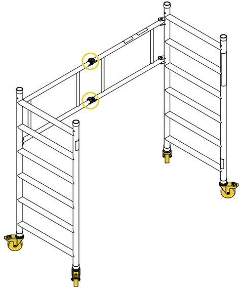
**2** Fit horizontal brace in position shown. Check tower is square and level.
