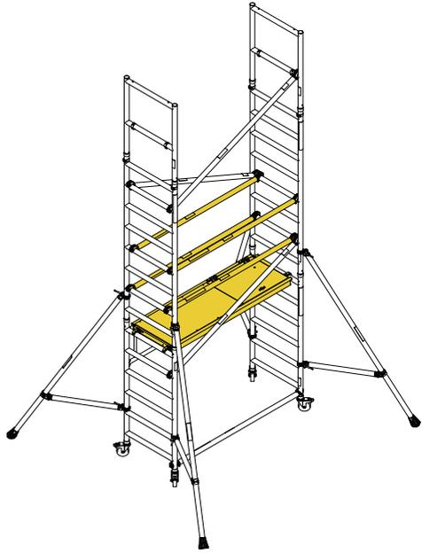
**10** Fit the trapdoor deck as shown. From the protected trapdoor position, fit horizontal braces as shown.
