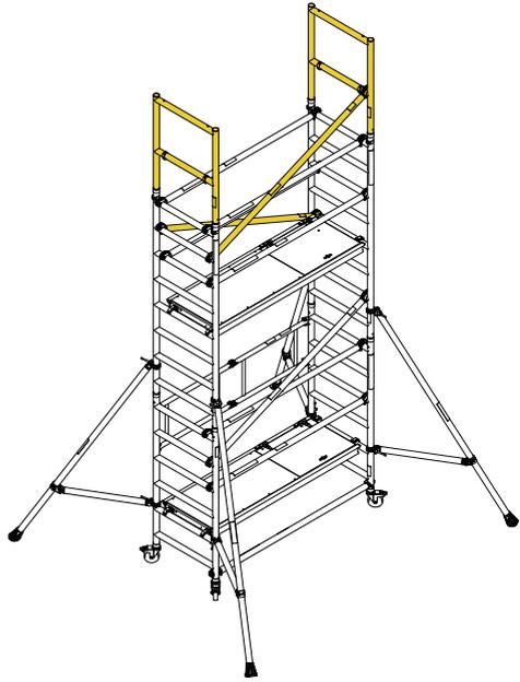
**8** Reposition trapdoor decks and horizontal braces.
